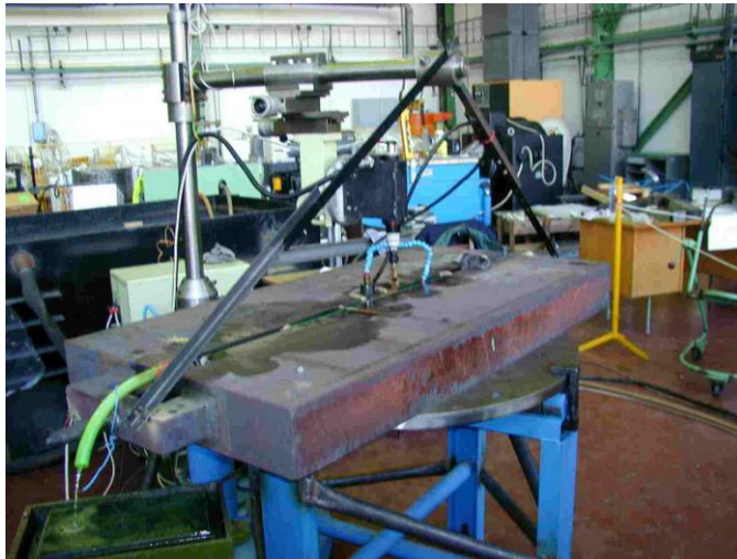
Fig. 1 - A phase of the manufacture of PISC type A defects into the WER 440 type RPV butt weld test assembly for open UT practical qualification trials
