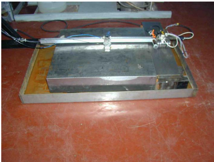
Fig. 2 - WWER 440 type RPV butt weld test assembly for open practical trials for UT qualification (dimensions 1450 x 790 x 140 mm)
