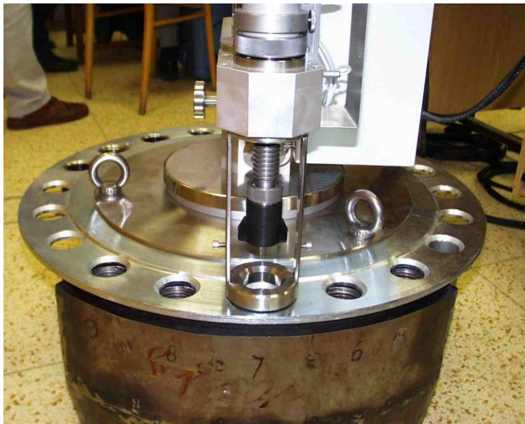
Fig. 3 - WWER 440 type SG collector thread holes test assembly with intended IGSCC type defects and EDM notches for open practical trials for UT and ET qualification
