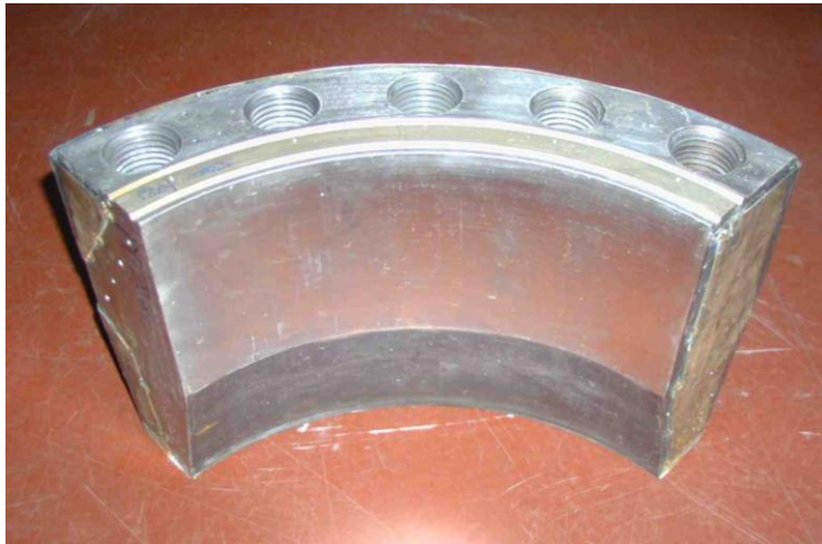
Fig. 3 - WWER 440 type SG collector thread holes test assembly with intended IGSCC type defects and EDM notches for open practical trials for UT and ET qualification
