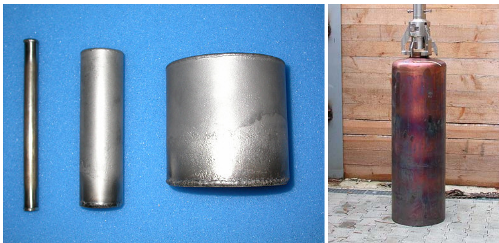
Fig. 1: Clad small scale glass specimen (left), real scale glass canister with lifting unit (right)
