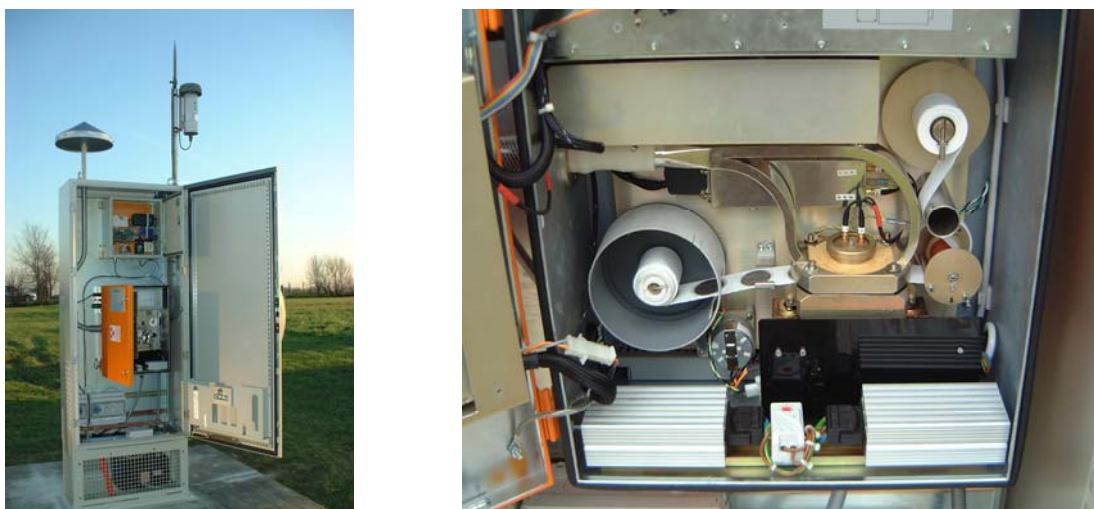
Figure 3 : Aerosol monitor (exterior and interior view of the monitor)
