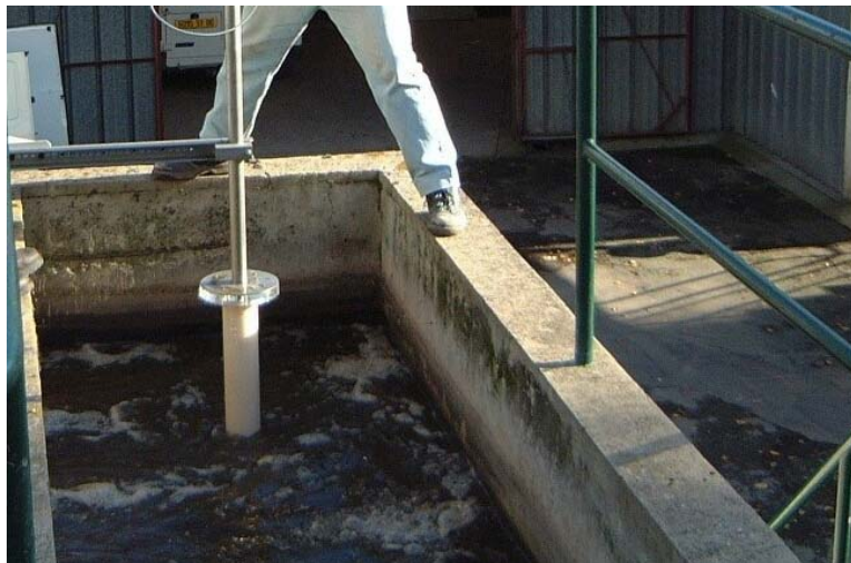
Figure 4 : Probe dedicated to the nuclear medicine wastes
