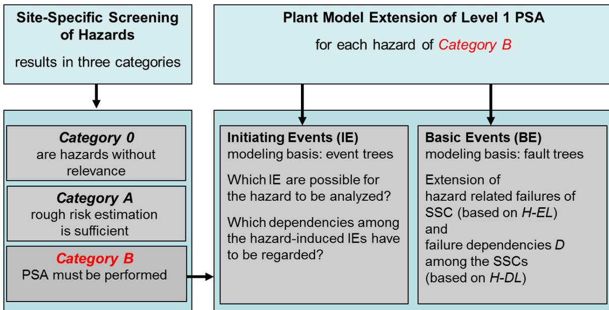
Figure 1: Structure of a Hazards PSA
