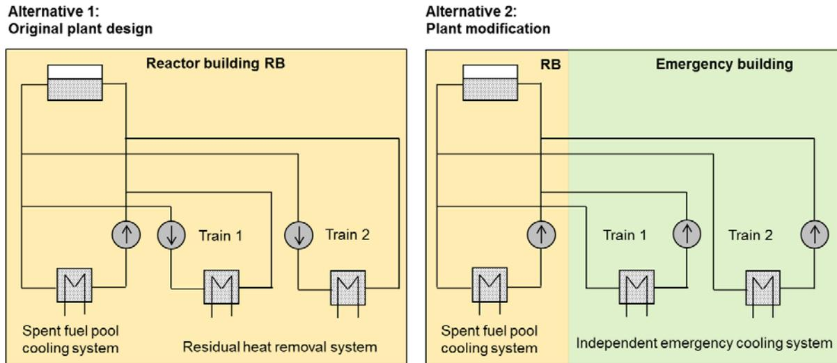
**Figure 3:** Alternatives of spent fuel pool cooling
