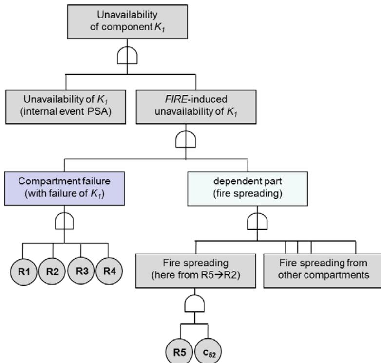
**Figure 4:** Fault tree extension using *F-EL* und *F-DL* in case of the internal hazard fire (exemplary component  $K_1$ )
