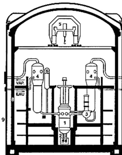
**Figure 4: schematic view of a French 1300 MWe PWR horizontal floors surrounding the reactor cavity**
