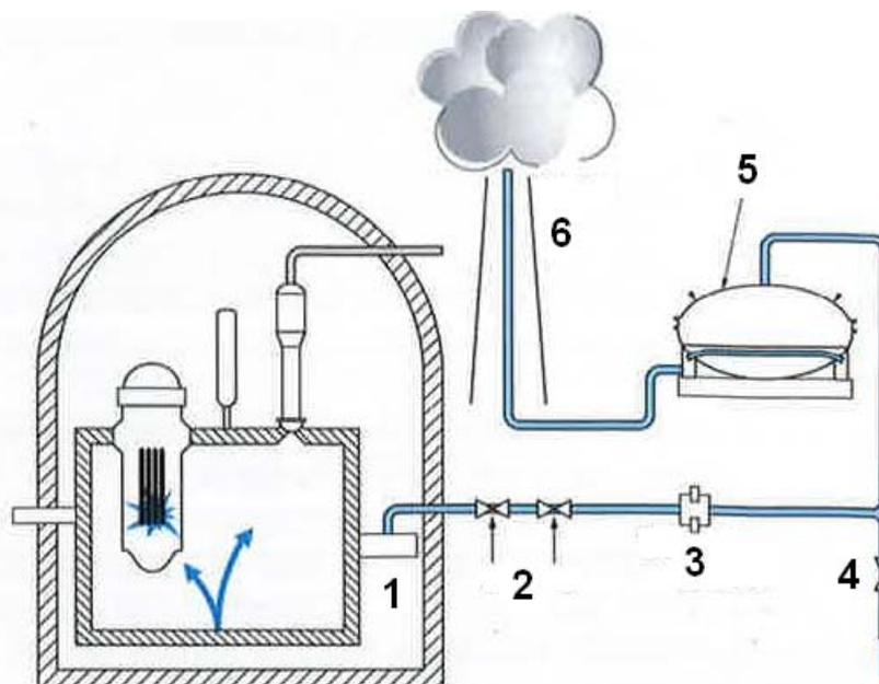
**Figure 5: schematic view of the French 1300 MWe PWR EFCVS**
