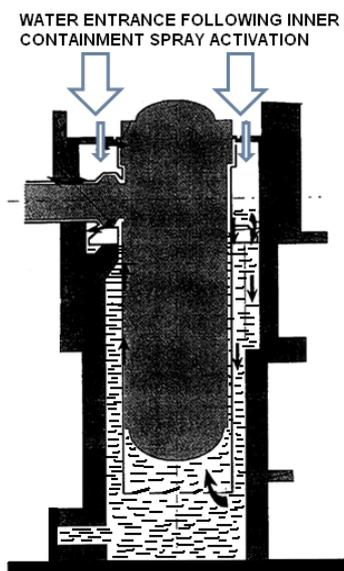
Figure 1: reactor cavity passively flooded up to the maximum level available (schematic view)
