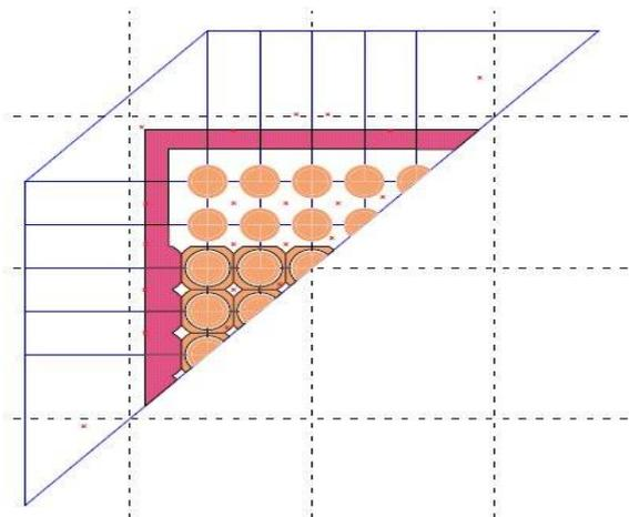
Figure 6. Modeling of half a FEBA test section with DRACCAR
