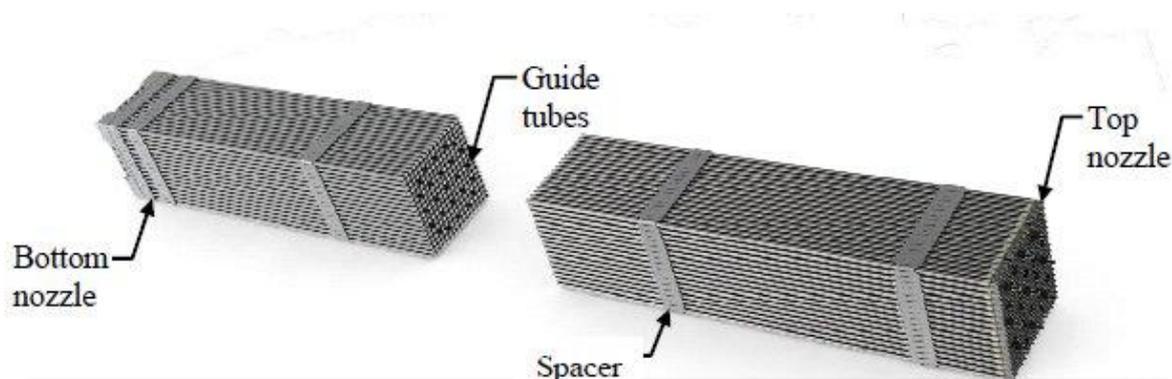
Figure 9. Various components in a typical 17x17 PWR fuel assembly
