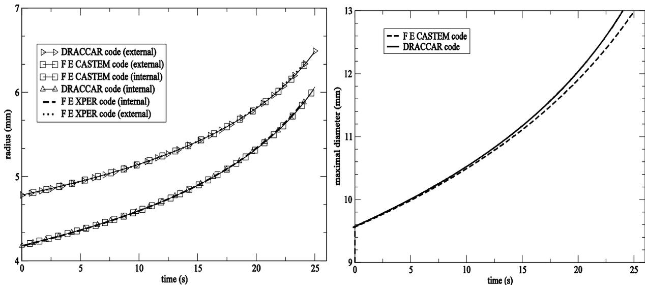
Figure 1. Numerical comparisons with FE computations. (left: test-case 1): internal and external radii evolutions for axi-symmetric loading; (right: test-case 2) : maximal diameters evolutions for azimuthal non-uniformities in temperature
