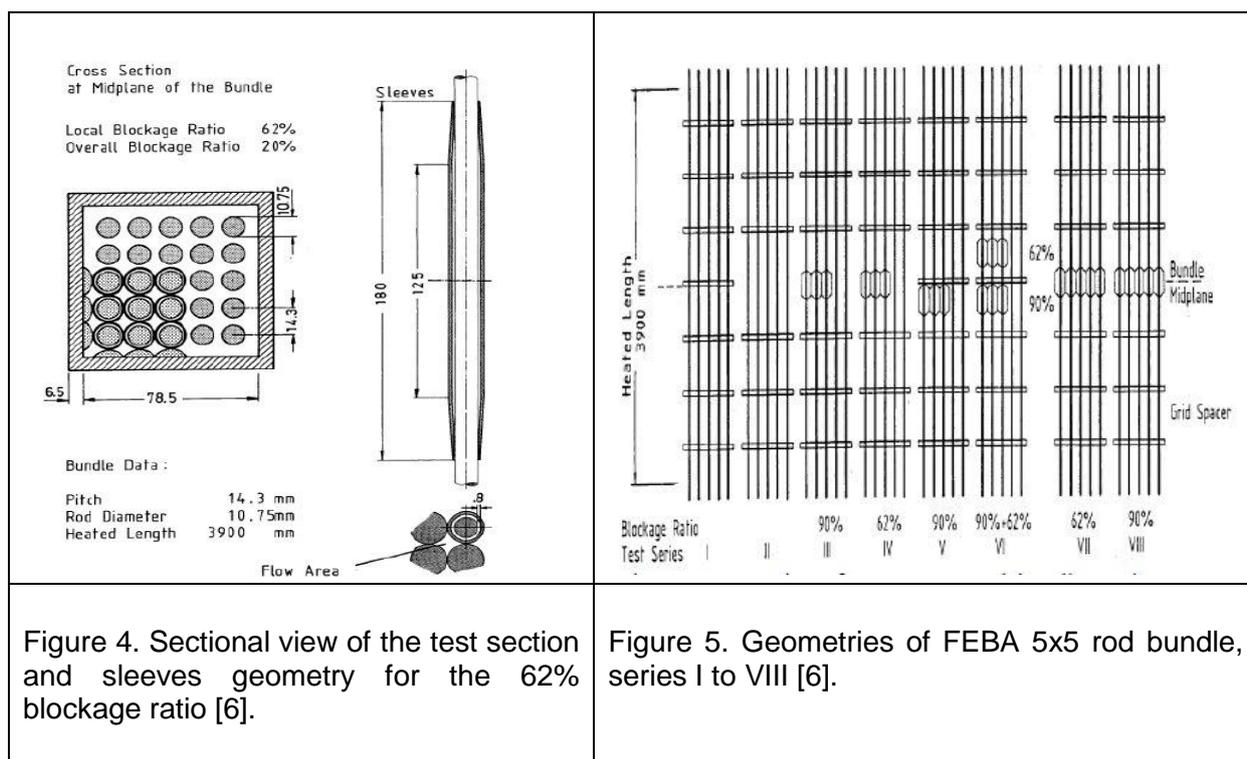
Figure 4. Sectional view of the test section and sleeves geometry for the 62% blockage ratio [6].
