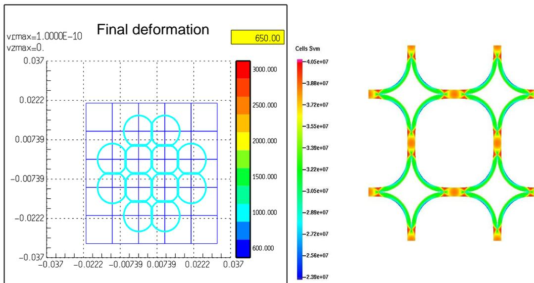
Figure 2. Test-case 3: left: DRACCAR view of the deformed bundle; right: the equivalent stress iso-values computed by the XPER code
