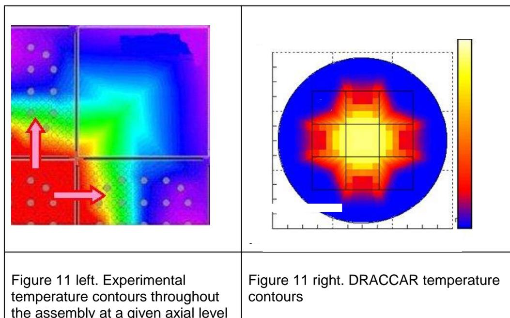
This specific geometry can be modelled using axis-symmetric codes but at the cost of some simplifying hypotheses to reproduce at best average experimental values. However, in order to get some “correct” code results, parametric tunings are necessary to fit at best the experimental results.
